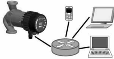
Figure 6: connecting to a network via router
